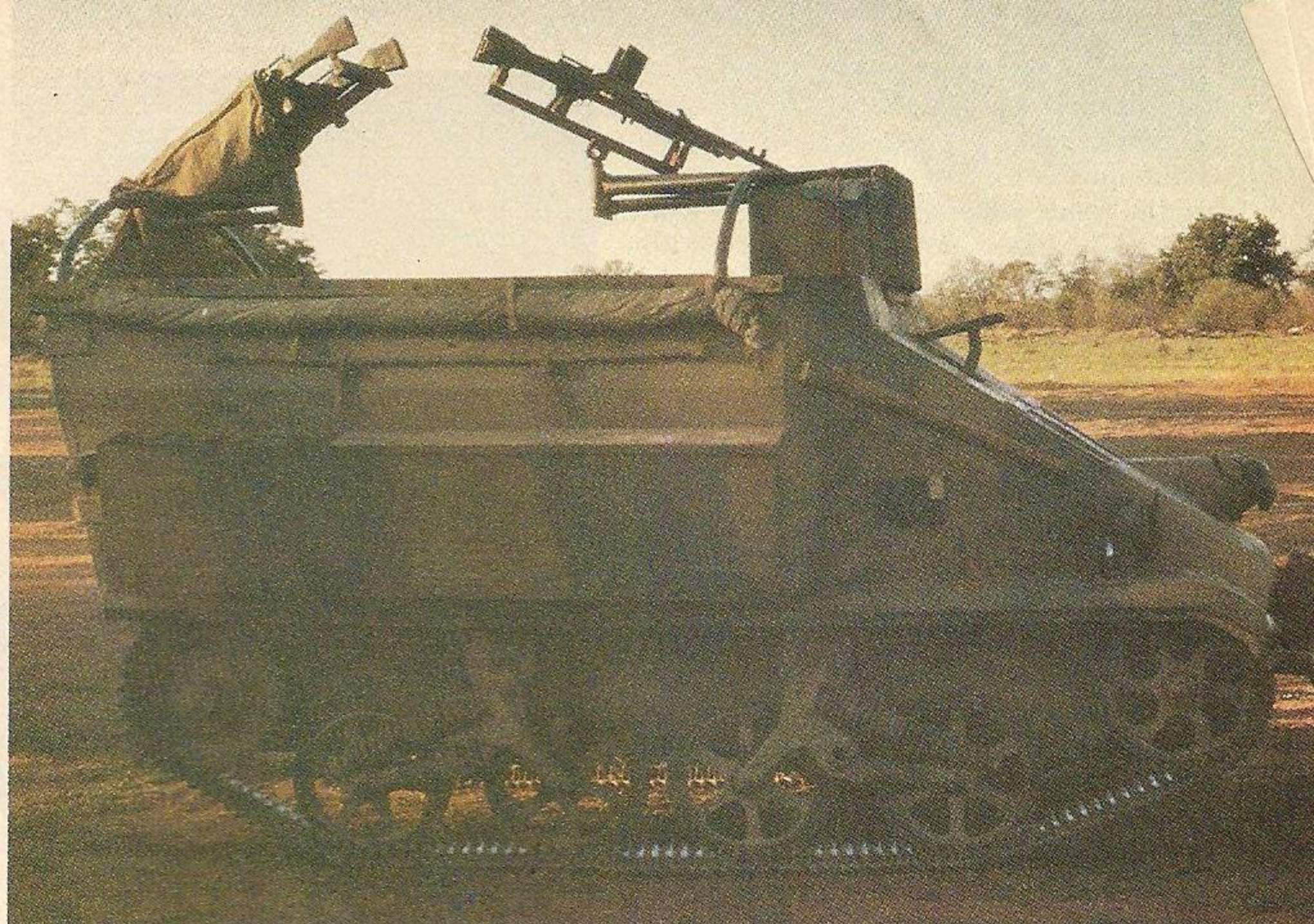
"War on a shoe-string." Rhodesian army is using WW-II Bren gun carrier with four MAG 7.62 machine guns for bush convoy protection.
